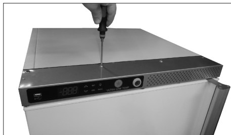
44. Remount the four topscrews
