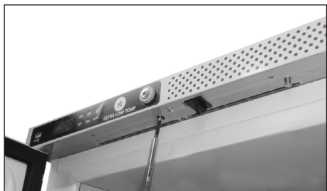
43. Remount the lock pin
