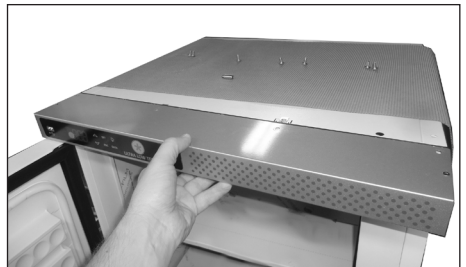
40. Carefully push the toppanel back into position
