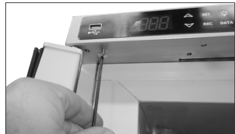
42....and remember the screw close to the top door pivot is mounted in hole nr.2 inwards, to ensure sufficient space between the screw and the door end-cap during mounting
