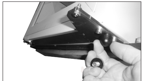
18. Remove the two front feet
