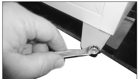
24. Remount and tighten pivot nut
