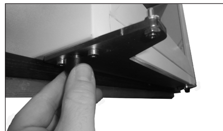
30. Remount and tighten the two front feet
